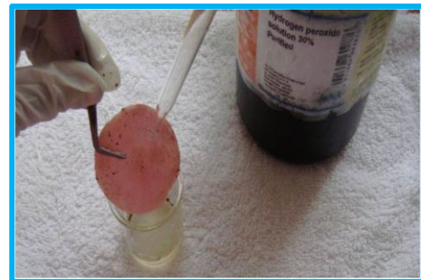
Fig. 4: Leaching of samples using 30% H 2 O 2
